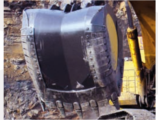
Patent-pending inverted keel reduces wear on the bottom of the bucket, enabling function without heavy wear package underneath.
