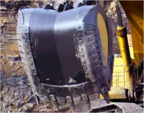
Patent-pending inverted keel reduces wear on the bottom of the bucket, enabling function without heavy wear package underneath.
