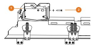
Inspect the bolts (Pos 1, 2) (3+3 nuts and bolts) on the Cradle bracket. If a bolt needs to be tightened, use a torque wrench to apply a torque to  $192 \pm 5$  Nm on the M14 (10.9) bolt from the outside of the Cradle bracket and use a wrench on the inside to hold the bolt back. (weekly basis)
