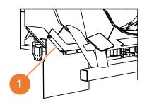
a) Inspect the Mudflap Plate bolts for damage (Pos. 1). Verify that no bolts are missing and that they are tightened.
