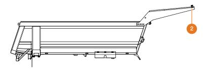
a) Inspect the Canopy Marker Lamps on both sides of the tipper body for damage and verify that they are functioning (Pos. 2).
