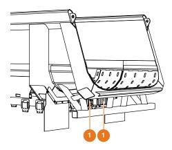
a) Inspect the Rear Lamps for damage and verify that they are functioning (Pos. 1).
